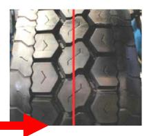
Laser marking line made on center of tread by Applicator – used as reference by Applicator to apply tread on casing centerline
